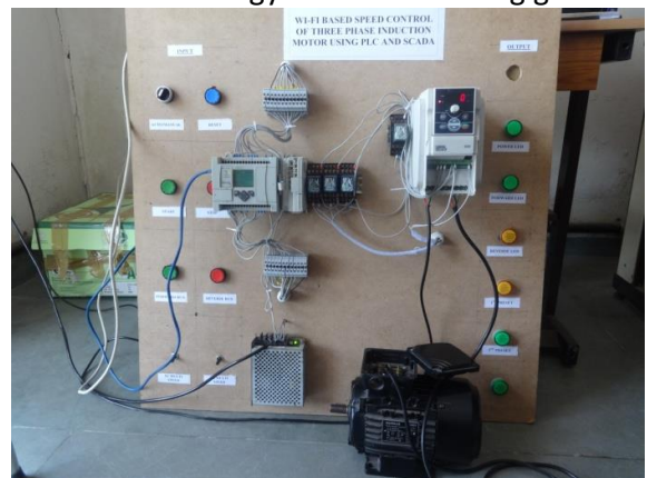
Wi-Fi BASED SPEED CONTROL OF 3-PHASE INDUCTION MOTOR THROUGH PLC AND SCADA
