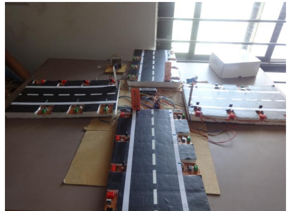
Intelligent Traffic Light And Density Control Using IR Sensors And Microcontroller
