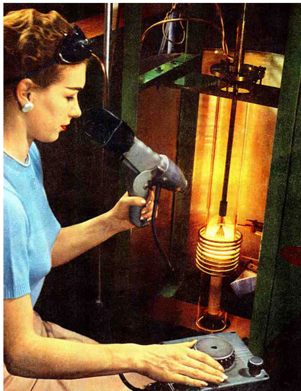
Figure 1.1: Czochralski setup for growth of 1 cm diameter silicon crystal used in 1956 [15].
