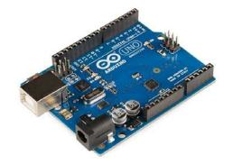
Arduino is an open-source physical computing platform based on a simple microcontroller board, and a development environment for writing software for the board. Arduino can be used to develop interactive objects, taking inputs from a variety of switches or sensors, and controlling a variety of lights, motors, and other physical outputs. Arduino projects can be stand-alone, or they can communicate with software running on your computer (e.g. Flash, Processing, MaxMSP.)
